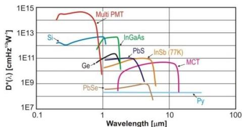
Fig. 1. Example of photodetectors detectivity [4]
