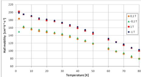
Fig. 1. The examples of temperature dependence of the Hall mobilities for the sample number 3704 for four values of magnetic field
