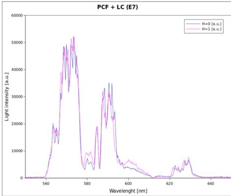
Fig. 2 Propagation spectras for photonic crystal fiber filled with liquid crystal under influence of external magnetic field
