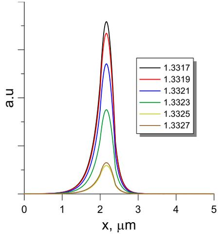
Fig.3. Optical signal at the output of single-mode waveguide for the refractive indices of the cover in the limit of 1.3317-1.3327.
