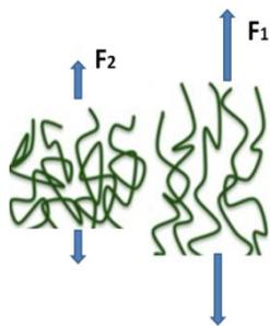
Fig. 1 Mechanism of "stretching" PMMA chains during the fiber drawing process ( $F_2 \gg F_1$ ).
