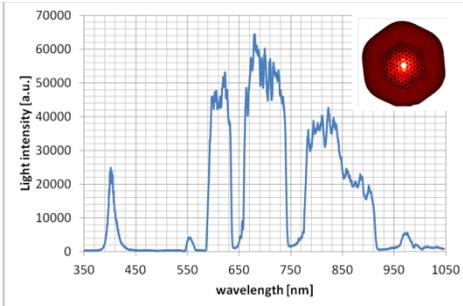
**Fig. 2** Halogen lamp spectrum in LMA-10 PCF infiltrated with 5721 azo-LC after illumination with UV light (*cis*-isomerization)
