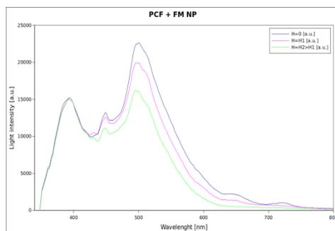
Fig. 1 Propagation spectras for photonic crystal fiber filled with ferromagnetic particles under influence of external magnetic field
