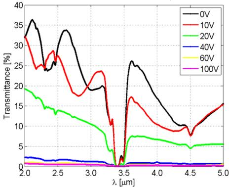
Fig. 2. Transmittance of TN modulator for different voltages.
