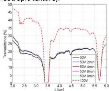
Fig. 1. Transmittance of ChLC modulator switched between focal conic and homeotropic texture by using 50 V and 120 V respectively
