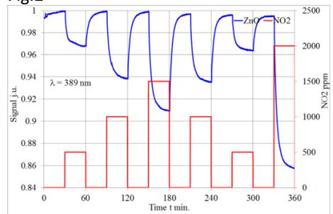
Fig. 2. Spectral transmission of ZnO under influence of  $\text{NO}_2$  gas environment.
