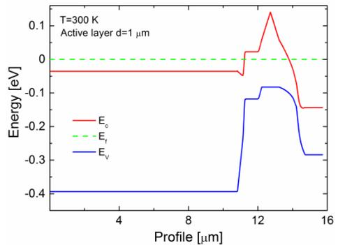
Fig. 1. Energy band diagram of the structure for ultra fast response time at 300 K
