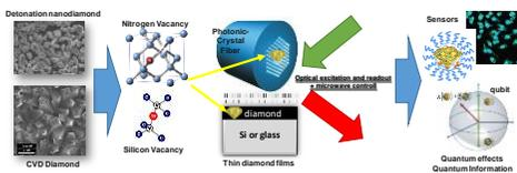
Fig. 1. The photonic and quantum devices based on color centers in diamond.
