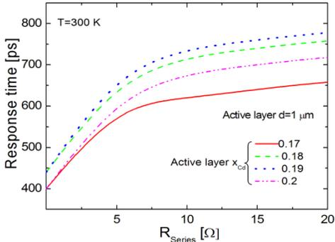
Fig. 2. Response time versus extra  $R_{Series}$  for selected active layer  $x_{Cd}$  at 300 K
