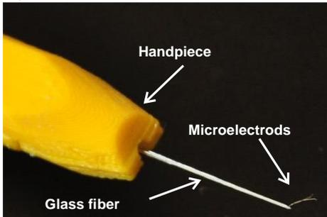
Fig. 2. Thin microprobe for electroporation of single cells.
