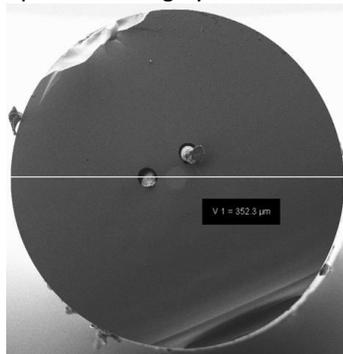
Fig. 1. Glass fiber with two low-resistant silver-copper microelectrodes, separated 31  $\mu\text{m}$  from each other, each with a diameter of 23  $\mu\text{m}$ .
