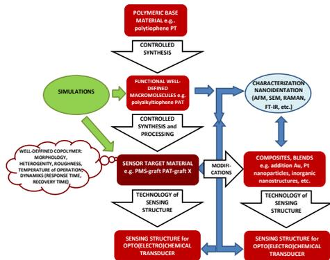
Fig. 1. Scheme of the process of the obtaining of sensing structures with adjustable properties.
