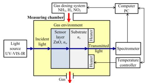
Fig. 1. Scheme of measurement setup.
