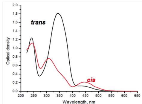
Fig.1. The absorbance spectrum of azo-LC 5721 (BEAM CO) in *trans*- and *cis*- forms.
