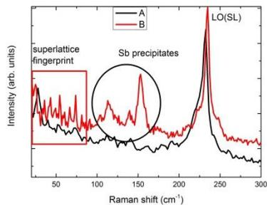
Fig. 2. Raman spectra of InAs/GaSb superlattice. For both samples superlattice fingerprint is marked by red rectangle, for
