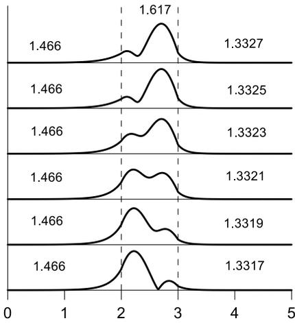
Fig.2. Amplitude distributions at the output of MMI section for the refractive indices of the cover in the limit of 1.3317-1.3327. Dotted lines denote the borders multimode waveguide.
