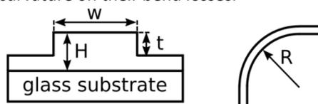
Fig. 1. Schematic of the rib waveguide,  $t$  - rib height,  $w$  - rib width,  $H$  - base slab thickness,  $R$  - radius of curvature.
