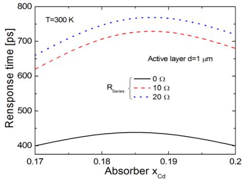
Fig. 3. Response time versus active layer  $x_{Cd}$  at 300 K
