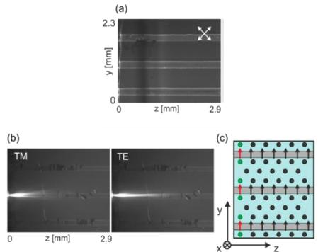
Fig. 1. a) Periodic structure obtained in NLC cell due to photo-polymerization process for the special mask applied and after irradiating the cell with UV light, as observed through crossed polarizers. (b) Propagation of low power beams with orthogonal polarizations when launched in the channels of planar orientation. (c) The scheme of photonic structure obtained thanks to the photo-polymerization process taking place in NLC layer.
