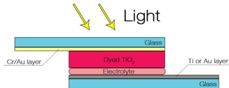
Fig. 1. Structure of elaborated DSSC.
