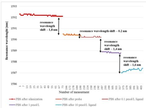
Fig. 1. Evolution of resonance the wavelength during each step of the biofunctionalization process, where: PBS – PBS after each step, probe – DNA ctivation step, specific DNA with concentrations: 0.1 pM, 1 pM, 10 pM.
