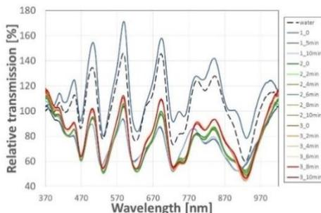
**Fig. 3.** Effect of the thin film electro-polymerization process on transmission of the sensor: transmission referred to response in air at different stage of the experiment and process time
