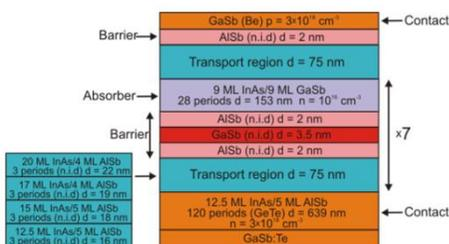
Fig. 1. Structural schematic of the MWIR T2SL cascade detector [after Ref. 1]
