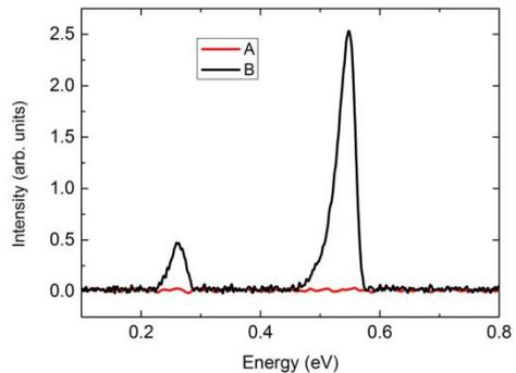
Fig. 1. Photoluminescence spectra of InAs/GaSb superlattice
