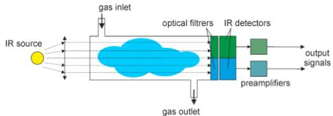
Fig. 1 NDIR sensor scheme.
