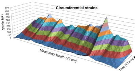
Fig. 1. A sample graph of obtained tensile strains of concrete specimen under test, in the time and distance domains [SHM System]
