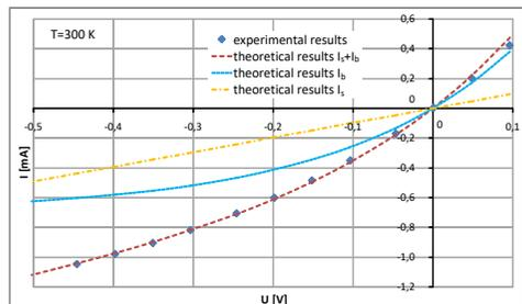
Fig. 2. Measured and modeled dark current versus bias voltage of T2SL InAs/GaSb cascade detector at 300K
