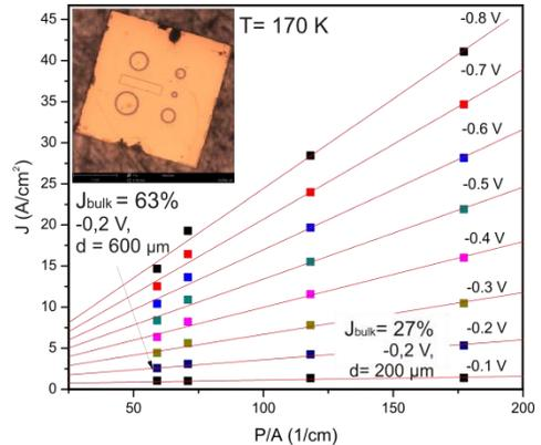
Fig. 1. The surface impact analysis on the unpassivated n<sup>+</sup>B<sub>p</sub>pN<sup>+</sup> HgCdTe structure
