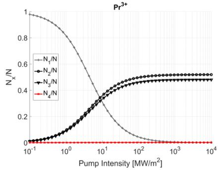
Fig. 2. Dependence of level populations on the pump intensity at pump wavelength of 1480 nm.
