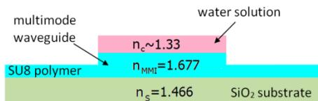
Fig.1. The geometry of one dimensional MMI structure in step-index configuration
