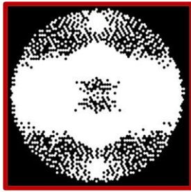
Fig. 2. The cross-section of the nanostructured five-mode fiber core (17,3 \mu\text{m} diameter) optimized using the convolutional neural network, along with the \text{Min}|\Delta n_{\text{eff}}| and bending losses values. Black dots and white dots correspond to silica glass rods and silica glass rods doped with 5 % mol of \text{GeO}_2 , respectively.
