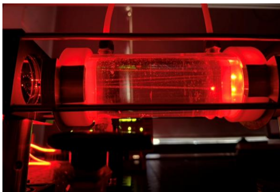
Fig. 3. Measurement chamber during calibration using a red laser (630 nm) – visible beam trajectory reflected between mirrors.
